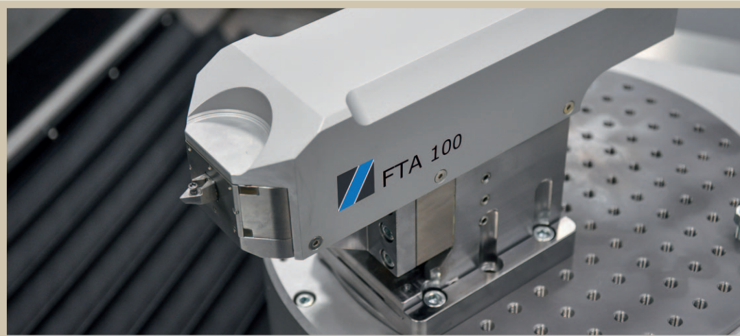
Figure 2. FTA100 piezo actuator based fast tool axis with 100 \mu\text{m} stroke for diamond machining of free-form surfaces and for micro and nano-structuring
