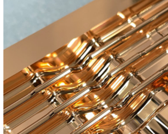
5-axis UP-milled particle accelerator component (CERN)
